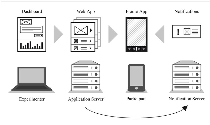
Fig. 1: Technical test setup during the Wizard of Oz phase
